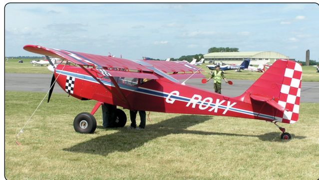
Figure 6-9. Flaperons on a Skystar Kitfox MK 7.
