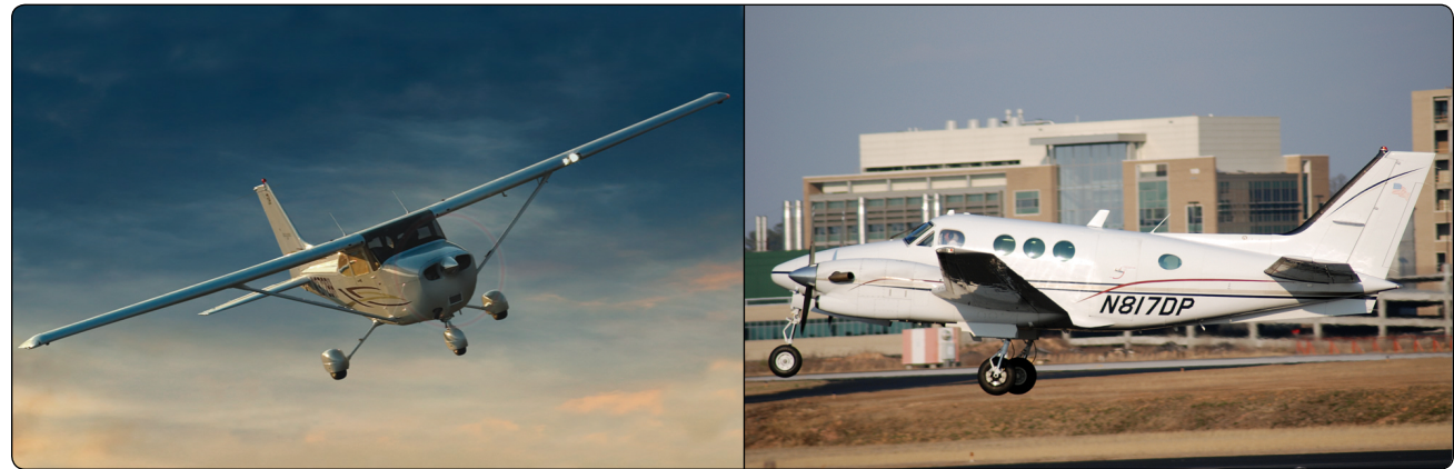
Figure 7-39. Fixed (left) and retractable (right) gear airplanes.
