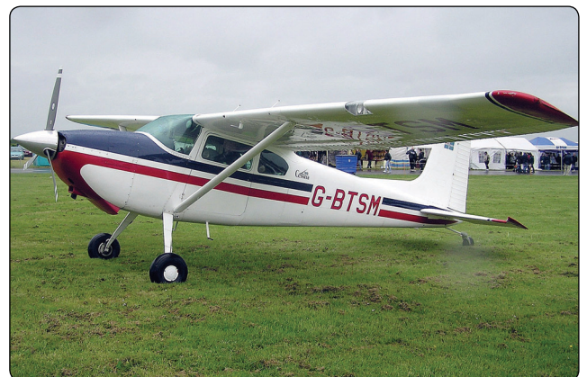
Figure 7-38. Tailwheel landing gear.
