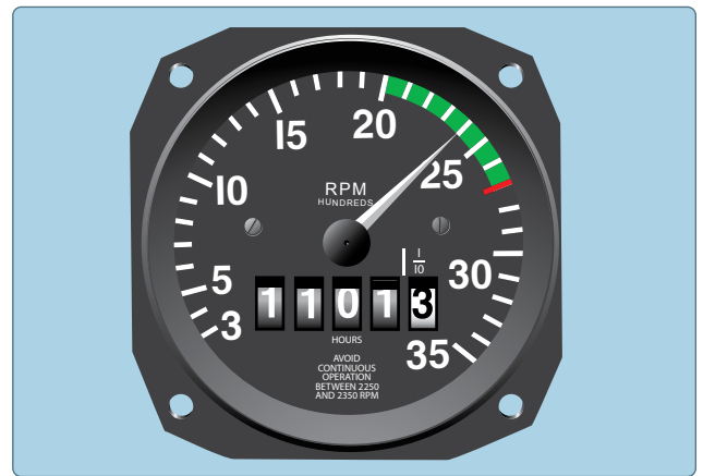
Figure 7-8. Engine rpm is indicated on the tachometer.
